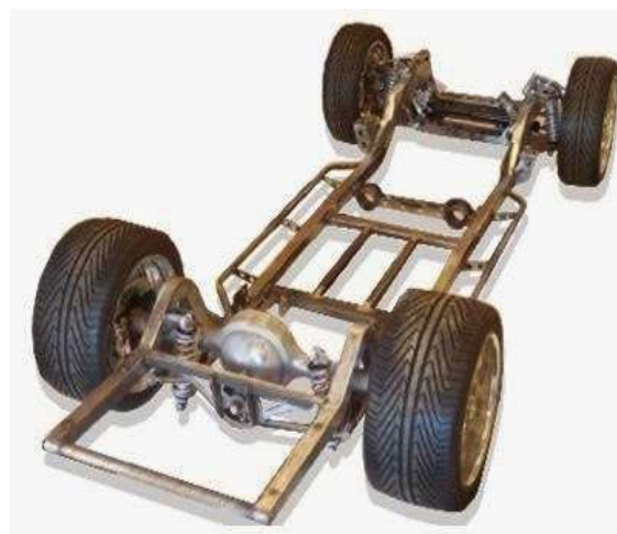
Fig.2.1. Conventional chassis or frame-full chassis.
